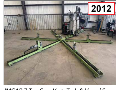
IMCAR 7-Ton Cap. Vert. Tank & Vessel Seam Welding System w/Fronius Dual-FCAW Full Penetration Welding
