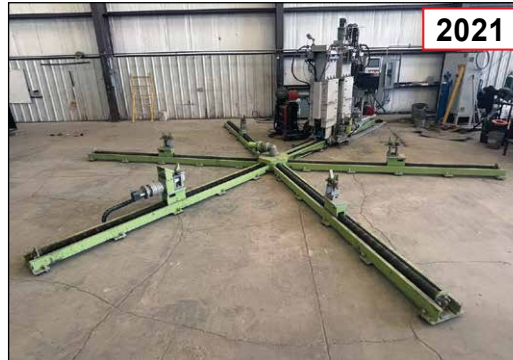
IMCAR 7-Ton Cap. Vert. Tank & Vessel Seam Welding System w/Fronius Dual-FCAW Full Penetration Welding
