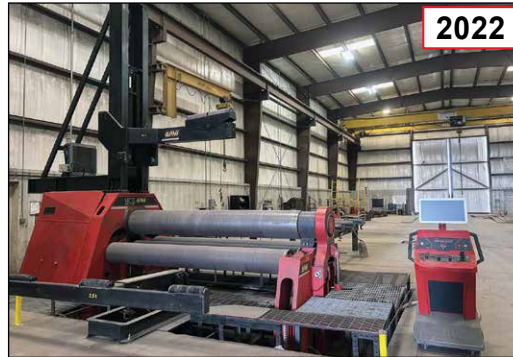
Davi 4-Roll 1-5/8" x 122" Cap. Model MCB i30 CNC Hydraulic Plate Bending Roll
