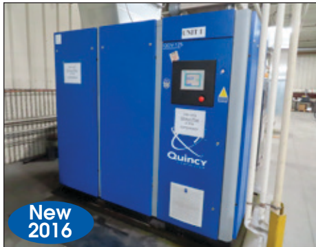
QUINCY 125 HP ROTARY SCREW AIR COMPRESSOR MODEL QGV-125
