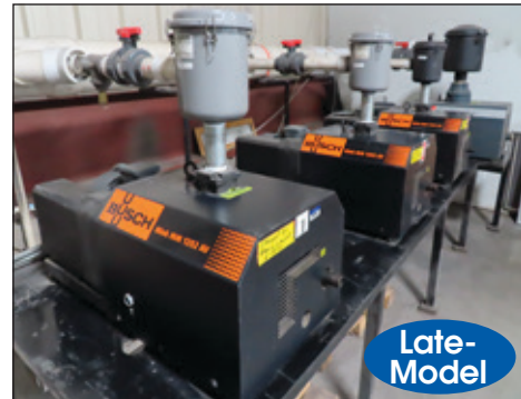
(5) BUSCH VACUUM PUMPS: MM1402AV & MINK MM1252AV
