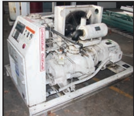
50HP Gardner Denver Rotary Screw Type Air Compressor
